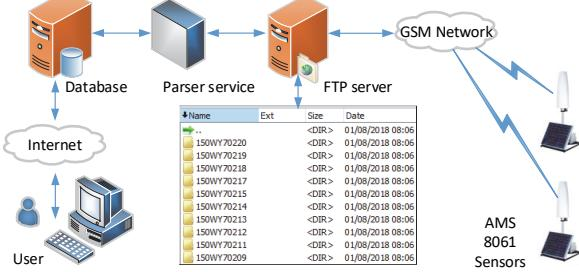
**Fig. 4.** The AMS 8061 data transfer in EMF RATEL system [11].
