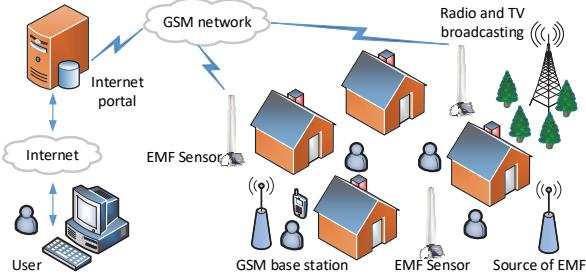
**Fig. 2.** The concept of EMF RATEL monitoring network.
