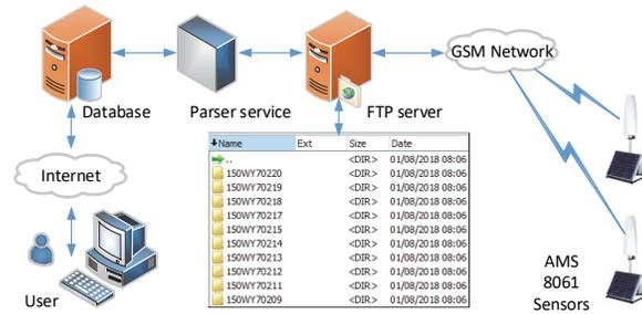
Fig. 4. The AMS 8061 data transfer in EMF RATEL system [11].
