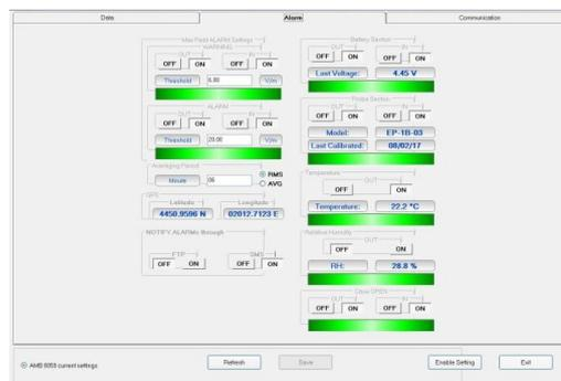
Figure 4. Defining the alarms that will be active on the sensor unit
