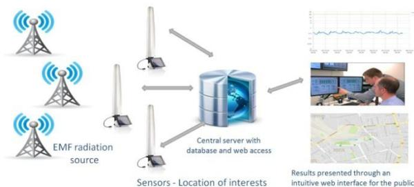
Figure 2. System architecture for continuous monitoring of the electromagnetic field level
